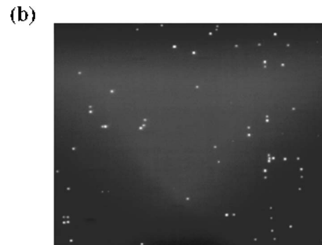
FIG. 3. (Color online) (a) TDD of the constant cap layers on graded SiGe buffers with and without thin strained layers (error bar shows \pm standard deviation) and (b) 210 \times 175 \mu\text{m}^2 dark field microscope image of control sample without thin strained layers after Secco etching.
